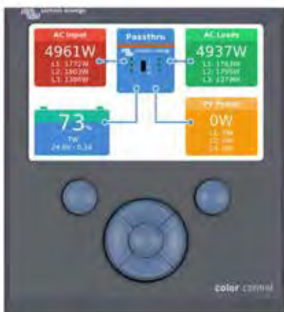
Color Control panel, showing a PV application
